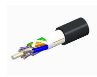
Fiber OSP cable, LazrSPEED® Single Jacket All-Dielectric, 96 fiber, Gel-Free, Stranded Loose Tube, Multimode OM3, Feet jacket marking, Black jacket color
