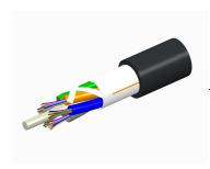
Fiber OSP cable, LazrSPEED® Single Jacket All-Dielectric, 144 fiber, Gel-Free, Stranded Loose Tube, Multimode OM3, Feet jacket marking, Black jacket color
