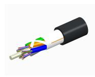
Fiber OSP cable, LazrSPEED® Single Jacket All-Dielectric, 288 fiber, Gel-Free, Stranded Loose Tube, Multimode OM3, Feet jacket marking, Black jacket color
