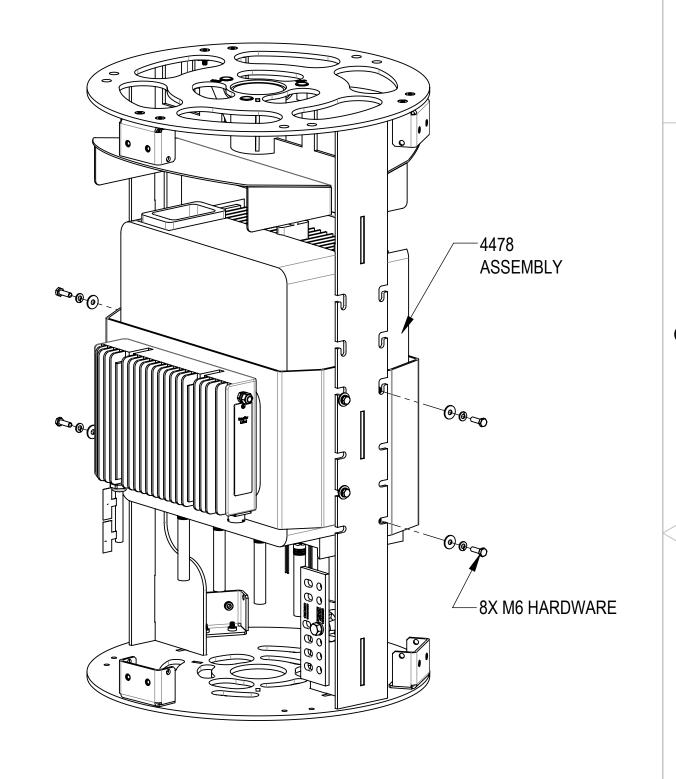
STEP 1: REMOVE TWO PRE-INSTALLED MOUNTING BRACKETS MTM1141-2000 AND MTM1141-3000, SAVE HARDWARE FOR STEP 2 AND STEP 3
