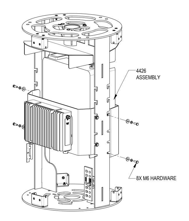
STEP 3 ( ALT 4426 ): INSTALL THE 4426-ASSEMBLY TO THE BRACKET OF POLE TOP USING 4 SETS OF TOP M6 BOLTS, LOCK WASHERS AND FLAT WASHERS
