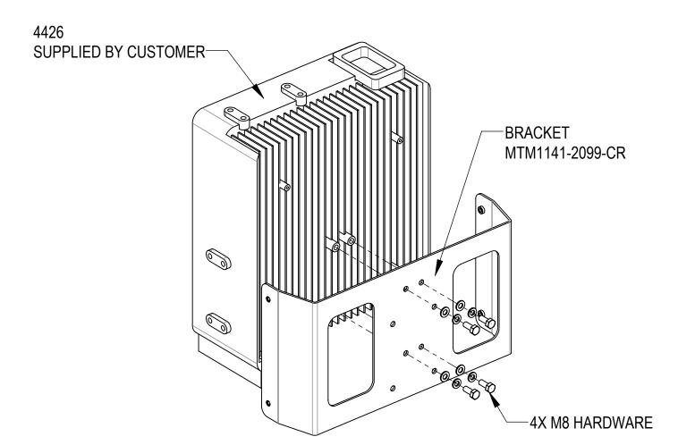
4426: INSTALL THE RADIO 4426 TO THE MOUNTING BRACKET MTM1141-2099-CR USING 4 SETS OF M8 SCREWS, LOCK WASHERS AND FLAT WASHERS AS SHOWN
