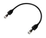
HELIAX® 1/2" Superflexible Fire retardant SureFlex® Jumper with interface types 7-16 DIN Male and 4.3-10 Male, 10M with black non-halogenated fire-retardant polyolefin jacket. with HELIAX® SureGuard weatherproofing..
