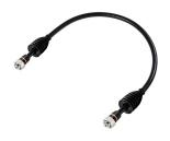
HELIAX® 1/2" Superflexible Fire retardant SureFlex® Jumper with interface types 7-16 DIN Male and 4.3-10 Male, 2M with black non-halogenated fire-retardant polyolefin jacket. with HELIAX® SureGuard weatherproofing.
