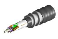
Fiber indoor/outdoor cable, TeraSPEED®, Plenum Rated, 144 fiber, Singlemode G.652.D and G.657.A1, Gel-Free, Stranded Loose Tube with Aluminum Interlocking Armor containing a Plenum Rated Outer Jacket, Black jacket color, Feet cable marking
