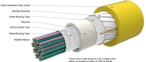
\*Picture shows cable design for 432F or higher where ribbons are bundled in groups of 144F per bundle. \*144F & 258F count designs use water blocking threads rather than a water blocking tape inside the buffer tube.
