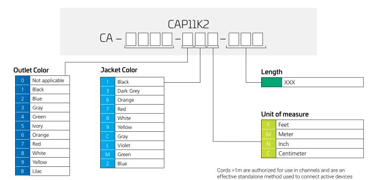
Cords < 1m are also valid elements for use in a channel or as an equipment interconnect but due to their limited lenght are not guaranteed to meet component compliance requirements that were developed to assess the quality of longer cords
