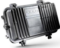
Flex Max® FM902 Broadband Trunk Amplifier, 1.2 GHz GaN output (equal trunk & bridger output tilt), 42-54 MHz Bandpass split, 27 dB Upstream gain, Full station, 40-90 Vac Powering
