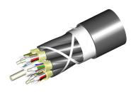
Fiber Indoor/Outdoor cable, TeraSPEED® Low Smoke Zero Halogen Riser Distribution, 48 fiber multi-unit with 12 fiber subunits, Gel-free, Singlemode + Multimode OM4, Feet jacket marking, Black jacket color, Cca flame rating
