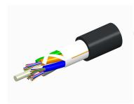
Fiber indoor/outdoor cable, TeraSPEED®, Single Jacket All-Dielectric (LSZH), 144 fiber, Singlemode G.652.D and G.657.A1, Gel-Free, Stranded Loose Tube, Black jacket color, Feet cable marking, Eca flame rating
