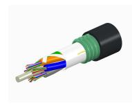
Fiber indoor/outdoor cable, TeraSPEED®, Single Jacket/Single Armor, Low Smoke Zero Halogen (LSZH), 24 fiber, Singlemode G.652.D and G. 657.A1, Gel-Free, Stranded Loose Tube, Black jacket color, Feet jacket marking
