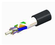
Fiber OSP cable, TeraSPEED® Single Jacket All-Dielectric, Gel-Free, Stranded Loose Tube, 18 fibers, Composite OM4 and G.652.D and G.657. Al, Feet jacket marking, Black jacket color
