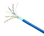
GigaSPEED X10D® 2291B ETL Verified Category 6A F/UTP Cable, plenum, blue jacket, 4 pair count, 1000 ft (305 m) length, reel
