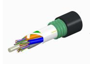
Fiber OSP cable, TeraSPEED® Single Jacket/Single Armor, 72 fiber, Gel-Free, Stranded Loose Tube, Singlemode G.652.D and G.657.A1, Meters jacket marking, Black jacket color
