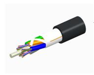
Fiber OSP cable, TeraSPEED® Single Jacket All-Dielectric, Gel-Free, 48 fibers, Stranded Loose Tube, Composite OM3 and G.652.D and G.657.Al, Feet jacket marking, Black jacket color
