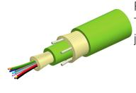
Fiber Indoor Cable, LazrSPEED® Low Smoke Zero Halogen Riser MPO Trunk Cable, 12 fiber, Gel-free, Multimode OM5, Dca Flame Rating, Feet jacket marking, Lime green jacket color
