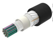
Fiber indoor/outdoor cable, All-Dielectric, LSZH Riser-Rated, Gel-Free, Central Tube Rollable Ribbon, 576 fiber, Singlemode G.657.A2/B2, Feet jacket marking, Black jacket color, Cca flame rating
