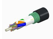
Fiber indoor/outdoor cable, TeraSPEED®, Single Jacket/Single Armor, Low Smoke Zero Halogen (LSZH), 6 fiber, Singlemode G.652.D and G. 657.A1, Gel Filled , Stranded Loose Tube, Meters jacket marking, Black jacket color, B2ca flame rating
