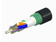
Fiber indoor/outdoor cable, TeraSPEED®, Single Jacket/Single Armor, Low Smoke Zero Halogen (LSZH), 96 fiber, Singlemode G.652.D and G. 657.A1, Gel Filled , Stranded Loose Tube, Black jacket color, Meters jacket marking, Cca flame rating
