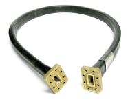
FlexTwist® Flexible Twist for WR112, 7.125–8.5 GHz, with interface types PBR84 and PBR84, 600 mm
