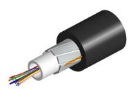
Fiber Indoor/Outdoor Drop Cable, LazrSPEED®, Low Smoke Zero Halogen Single Jacket All-Dielectric Arid-Core, 6 fiber, Gel-filled, Multimode OM3, Feet jacket marking, Black jacket color, Dca flame rating
