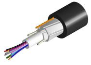
Fiber Indoor/Outdoor Drop Cable, LazrSPEED®, Low Smoke Zero Halogen Single Jacket All-Dielectric Arid-Core, 12 fiber, Gel-filled, Multimode OM3, Feet jacket marking, Black jacket color, Dca flame rating
