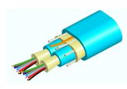
Fiber indoor cable, LazrSPEED®, Low Smoke Zero Halogen Riser MPO Trunk, 24 fiber with 12 fiber subunits, Gel-free, Multimode OM3, Feet jacket marking, Aqua jacket color, Dca flame rating
