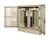
FDH 3000 Fiber Distribution Large Cabinet, 576F, SC/APC,(2) 32-splitter modules, single armor loose tube, 100 ft, 24F
