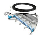
MFPS Fiber Optic panel, 1RU, 96 fibers/RU, pre-cabled I/O LSZH, 10m, front patch cords orientation to the left, 96 LC/UPC, grade C
