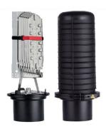
FOSC® 450 C6 Fiber Optic Splice Closure, Gel Cable sealing, two preinstalled 12-splice tray, 6 cable attach., no ground feedthrough lugs, with test valve
