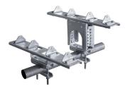
Side-By-Side Mounting Kit to mount two antennas on a pipe with 2.375 - 4.5 inch (60 – 115 mm) diameter
