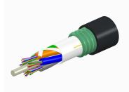
Fiber indoor/outdoor cable, TeraSPEED®, Mini Single Jacket,CST Armor, LSZH, 120 fiber, Gel-Filled, Stranded Loose Tube, Singlemode G.652.D and G.657.A1, Meters jacket marking, Black jacket color, Eca flame rating
