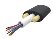
Fiber drop cable, Self-Supporting All-Dielectric, 12 fiber Arid Core construction, central loose tube, Gel-filled, Singlemode G.657.A2/B2, Feet jacket marking, Black jacket color, Build America Buy America (BABA)
