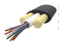
Fiber outdoor drop cable, LightScope® ZWP Self-Supporting All-Dielectric, Singlemode G.652.D and G.657.Al, 2 fiber Arid Core construction, Gel-filled, central loose tube, no ripcords, Feet jacket marking, Black jacket color
