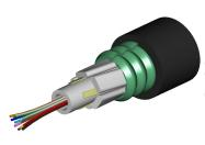
Fiber drop cable, LightScope ZWP® Single Jacket Single Armor Outdoor Drop Cable, 12 fiber Arid Core construction, central loose tube, Gel-filled, Singlemode G.652.D and G.657.A1, Meter jacket marking, Black jacket color
