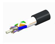
Fiber OSP cable, LightScope ZWP® Single Jacket All-Dielectric, 48 fiber, Gel-Free, Stranded Loose Tube, Singlemode G.652.D and G.657.A1, Feet jacket marking, Black jacket color
