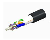
Fiber OSP cable, LightScope ZWP® Single Jacket All-Dielectric, 60 fiber, Gel-Free, Stranded Loose Tube, Singlemode G.652.D and G.657.A1, Feet jacket marking, Black jacket color
