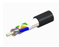
Fiber OSP cable, LightScope ZWP® Single Jacket All-Dielectric, 288 fiber, Gel-Free, Stranded Loose Tube, Singlemode G.652.D and G.657.A1, Meter jacket marking, Black jacket color
