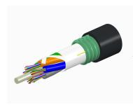
Fiber OSP cable, LightScope ZWP® Single Jacket/Single Armor, 18 fiber, Gel-Free, Stranded Loose Tube, Singlemode G.652.D and G.657.A1, Feet jacket marking, Black jacket color
