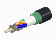
Fiber OSP cable, LightScope ZWP® Single Jacket/Single Armor, 16 fiber, Gel-Free, Stranded Loose Tube, Singlemode G.652.D and G.657.A1, Meters jacket marking, Black jacket color
