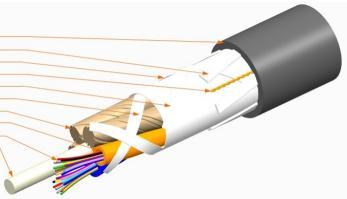
Plenum-Rated Outer Jacket Strength Elements Binder Water Swellable Tape Ripcord (1) Binder 2.5 mm Gel-Free Buffer Tubes 250 micron Fibers Dielectric Strength Member
