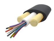
Fiber outdoor drop cable, LightScope ZWP® Self-Supporting All-Dielectric, Singlemode G.652.D and G.657.Al, 8 fiber Arid Core construction, Gel-filled, central loose tube, Meter jacket marking, Black jacket color
