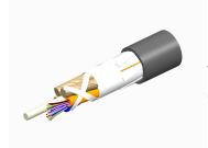
Fiber indoor/outdoor cable, LightScope ZWP®, Single Jacket All-Dielectric, Plenum Rated, Gel-Free, Singlemode G.652.D and G.657.A1, 36 fiber, Stranded Loose Tube, PVDF jacket, Feet jacket marking, Black jacket color
