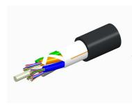
Fiber OSP cable, LightScope ZWP® Single Jacket All-Dielectric, 192 fiber, Gel-Free, Stranded Loose Tube, Singlemode G.652.D and G.657.A1, Meter jacket marking, Black jacket color
