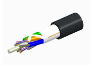
Fiber OSP cable, LightScope ZWP® Single Jacket All-Dielectric, 132 fiber, Gel-Free, Stranded Loose Tube, Singlemode G.652.D and G.657.A1, Meters jacket marking, Black jacket color
