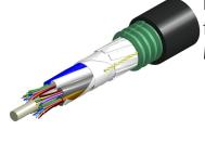
Fiber OSP cable, LightScope ZWP® Mini Single Jacket/Single Armor, 6 fiber, Gel-Filled, Stranded Loose Tube, Singlemode G.652.D and G.657.A1, Meters jacket marking, Black jacket color
