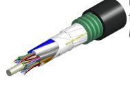
Fiber OSP cable, LightScope ZWP® Mini Single Jacket/Single Armor, 12 fiber, Gel-Filled, Stranded Loose Tube, Singlemode G.652.D and G.657.A1, Meters jacket marking, Black jacket color
