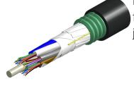
Fiber OSP cable, LightScope ZWP® Mini Single Jacket/Single Armor, 96 fiber, Gel-Filled, Stranded Loose Tube, Singlemode G.657.A2, Meters jacket marking, Black jacket color
