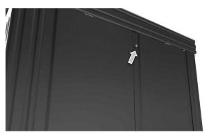
Use an Allan key  $n^\circ 5$  with conical head to fix the back panels with screws and washers (torque of 3.5-4Nm).
