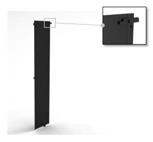
Place the rotating bracket in horizontal position.
