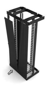
Place the positioning bracket at the bottom of the back panel in the horizontal groove of the NETpodium profile.
