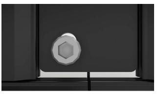
Use an Allan key n°5 with conical head to fix the back strip with screws and washers (torque of 3.5-4Nm).
