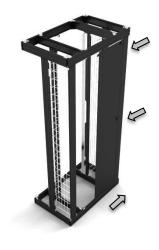
Slide the back panel to the right and insert the positioning brackets on the side of the back panel into the vertical groove of the NETpodium profile.
