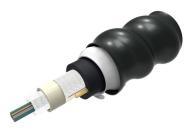
Fiber Indoor/outdoor Cable, Interlocking Armored, Low Smoke Zero Halogen (LSZH), Riser-Rated, 24 fiber, Gel-Free, Central Tube Ribbon, Singlemode G.652.D and G.657.A1, Feet jacket marking, Black jacket color
