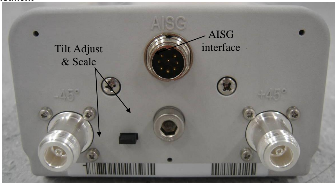
Figure 9. AISG Compliant Adjustable Downtilt Antenna showing Hex Socket for Manual Adjustment and Horizontal Angle Indicator Scale protruding past face of base.
