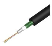
Fiber indoor/outdoor drop cable, LSZH, Gel-filled Central Tube, CST, 12 fiber, Singlemode G.652.D and G.657.A1, Meters jacket marking, Black jacket color
